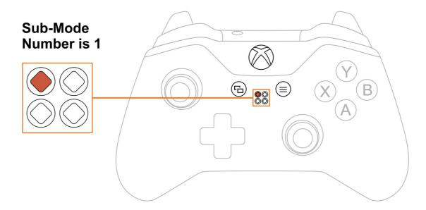
Upon checking the sub-mode, the modchip will automatically take you to the place you were before in 3 seconds. You are welcome to expedite the process by pressing the mod button on the back and exiting the sub-mode menu.
