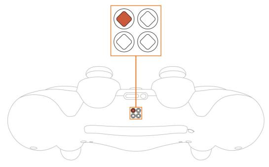
Upon checking the sub-mode, the modchip will automatically take you to the place you were before in 3 seconds. You are welcome to expedite the process by pressing the mod button on the back and exiting the sub-mode menu.
