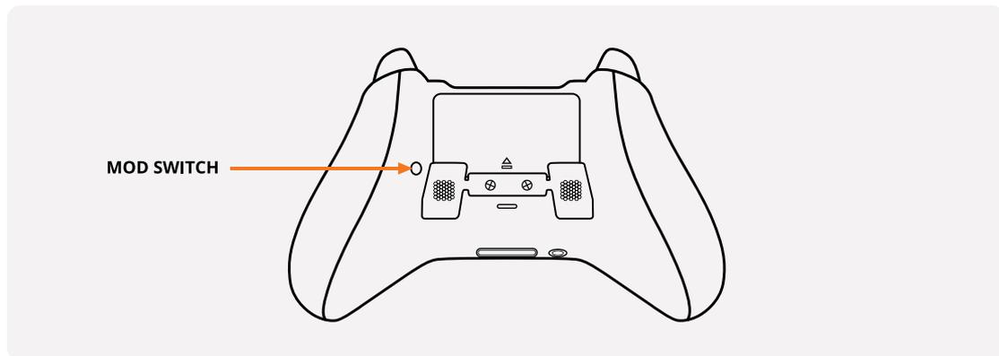
Holding down the mod switch will be your first step to perform any of these actions. You will always have to hold it down and then tap other corresponding buttons. Mod switch is only used for activating/deactivating modes, setting up custom setting and scrolling between sub-modes - you **DO NOT** have to press it for any other purposes during the game play.
